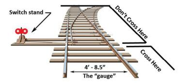
**6.0.4** Do not walk lengthwise between the two rails of a track (known as the "gauge" of the track) and <u>do not step on the actual rails.</u>
